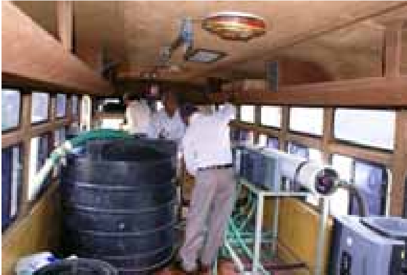
Mobile RO Desalination Plant
