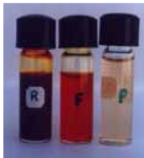
F: Initial feed P: final permeate after 80% recovery R: Concentrate Reactive red 2; Reactive red 120 Reactive orange 4; Reactive orange 13
