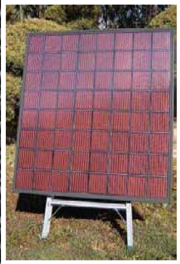
Series connected 64 DSC cells
